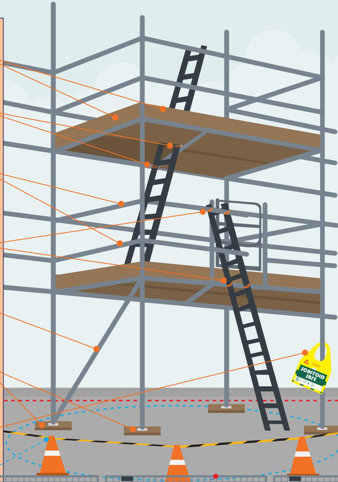
Exclusion zones are required if scaffold is installed for up to 24 hours. Cones and retractable bars or folding fences are sufficient, if the scaffold is under supervision.
